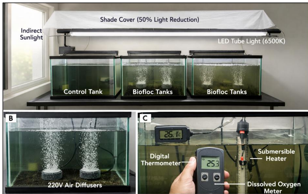
Figure 1. Experimental aquarium setup
