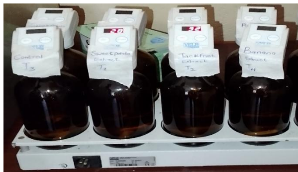
Figure 3. Determination of BOD in effluent water from tanks fed fermented ripe banana, jackfruit seeds, and sweet potato tubers, compared with the control feed
